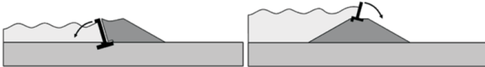
Figure 3.189 Tilting of walls in composite levee due to differential settlements (courtesy Y Deniaud, CETMEF)
