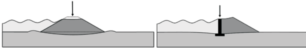
Figure 3.187 Settlement of a levee on a soft soil foundation (courtesy Y Deniaud, CETMEF)
