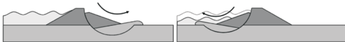
Figure 3.184 Deep rotational sliding of a levee (courtesy Y Deniaud, CETMEF)
