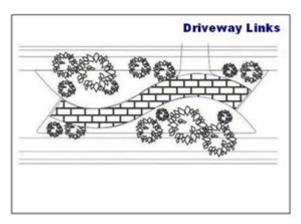
Driveway links introduce an effective one-way one-lane section of road to reduce speeds and discourage through traffic. They generally provide a greater visual and physical impact than slow points, but may restrict access for emergency vehicles and reduce on-street parking. This is not considered a cost-effective treatment due to the use of extensive infrastructure and landscaping, which also requires a higher degree of ongoing maintenance.
