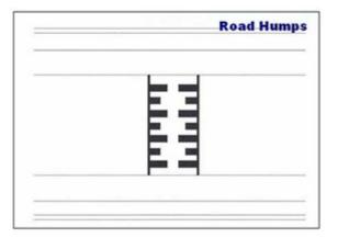
Road humps are a cost-effective treatment for lowering average traffic speeds; however they may negatively impact residents by increasing traffic noise and may cause an uncomfortable ride for vehicle passengers and cyclists. The installation of road humps also requires additional street lighting to illuminate the device, which may negatively impact adjacent residences.
