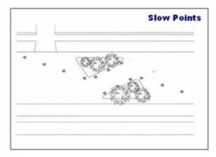
Slow points are a series of kerb extensions on opposing sides of the street to narrow and/or angle the road. They are quite effective in lowering average traffic speed, but may restrict access for emergency vehicles and require the removal of on-street parking.
