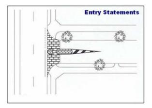
Entry statements are coloured and/or textured surface treatments placed at the entry of an LATM area to alert drivers that they are entering a driving environment that is different from the one they just left. They effectively constrain the throat of the intersection to lower average traffic speeds and discourage heavy vehicle entry. To be effective, this treatment should be supplemented by mid-block treatments, such as the three shown below.
