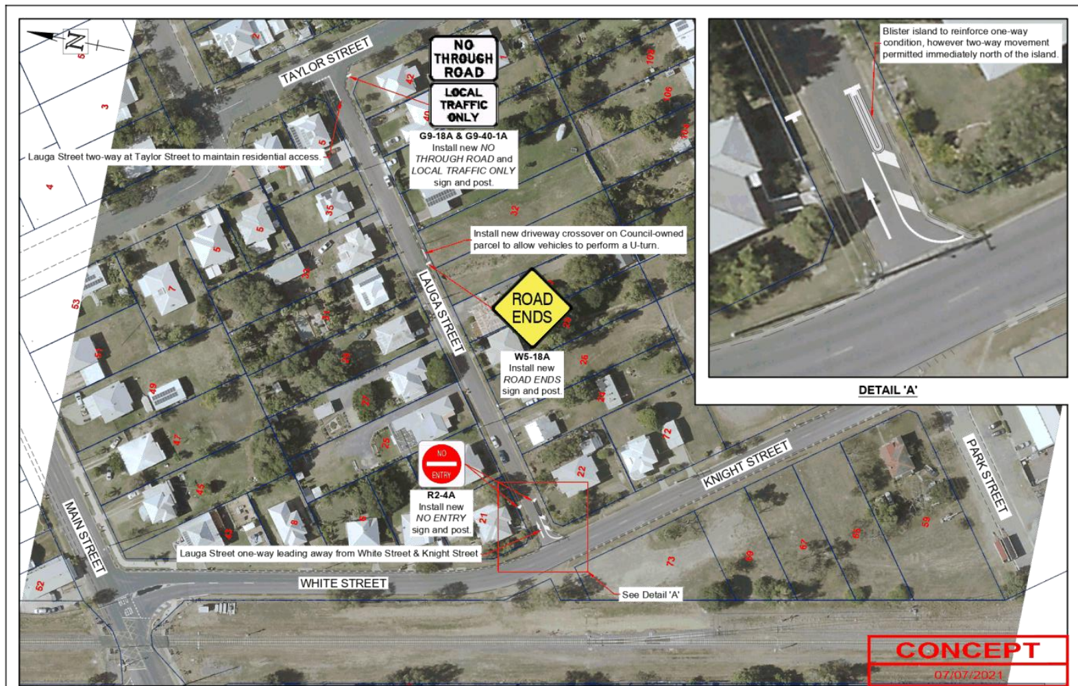
LAYOUT PLAN - OPTION C - ONE-WAY AWAY FROM KNIGHT STREET & WHITE STREET, TWO-WAY AT TAYLOR STREET ($9,000)
