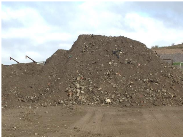
3 Oversize after Screening reading for crushing
