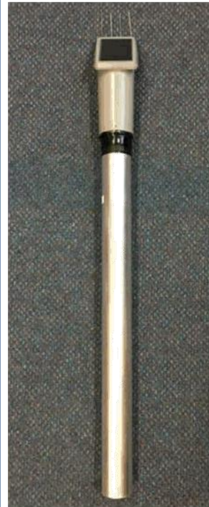
The ParkNet Relay – solar/battery device connecting DCA sensor to the DCA ParkNet wireless parking data network (post nominal bore dia = 50mm).
