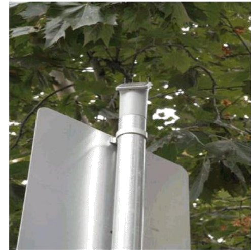
The ParkNet Relay – solar/battery device connecting DCA sensor to the DCA ParkNet wireless parking data network (post nominal bore dia = 50mm).
