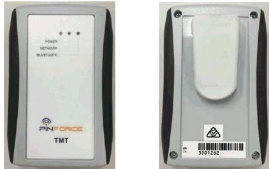
Pinforce TMT – standalone device bridges bluetooth communication between Local Laws PDA and the DCA sensor.
