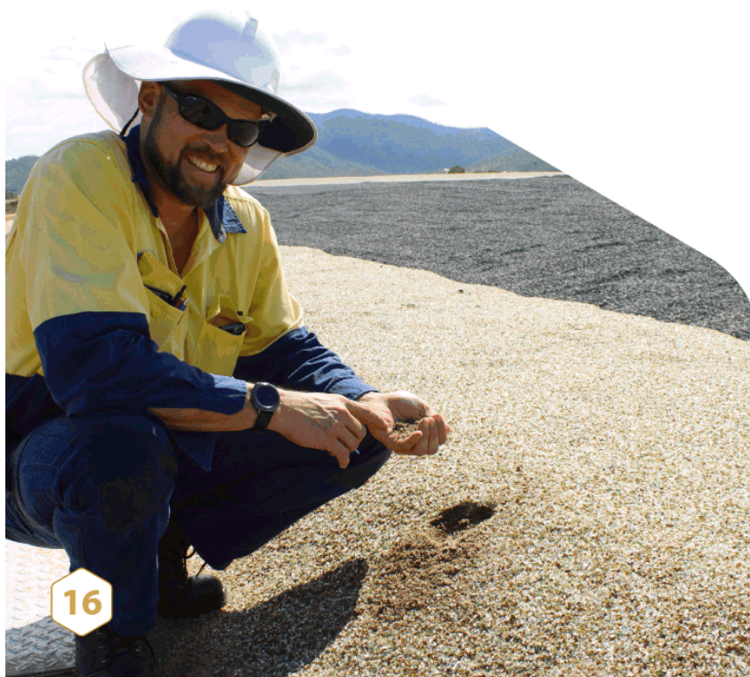
Rockhampton Regional Waste and Recycling has used crushed glass in place of sand in projects at the Lakes Creek Road Landfill.
