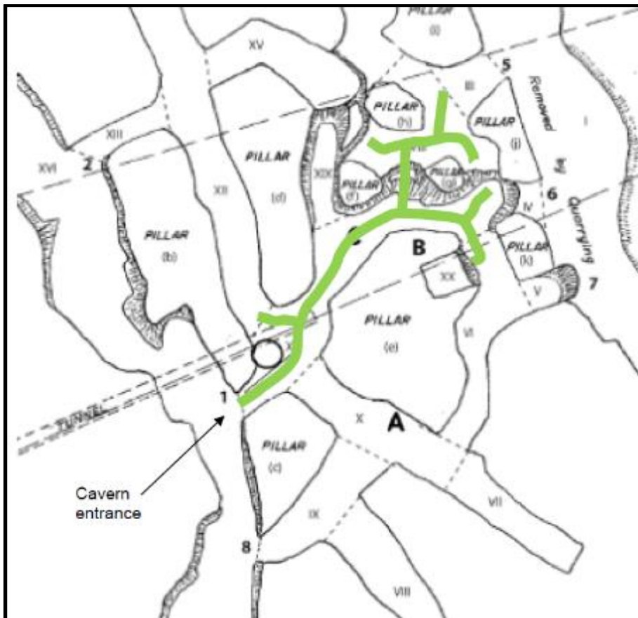
Figure 6-3 Recommended Bolts and Mesh (Golder, 2011a).
