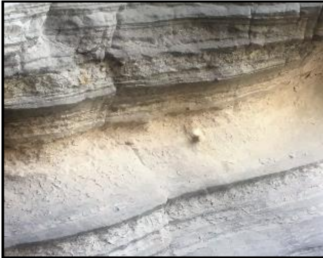
Figure 4-30 Example of an Erosion Pin.
