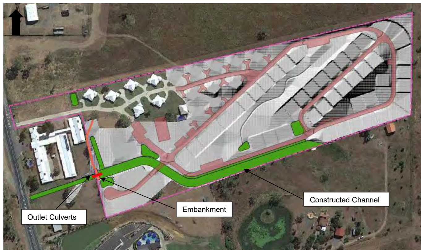
Figure 3-13: Constructed Channel and Embankment
