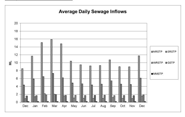
Average daily sewage inflows during December increased compared to that reported in November due to the receipt of significant rainfall in most locations during the month. The rainfall was sufficiently heavy to lead to increased flow to each STP through inflow and infiltration of the sewerage networks.
