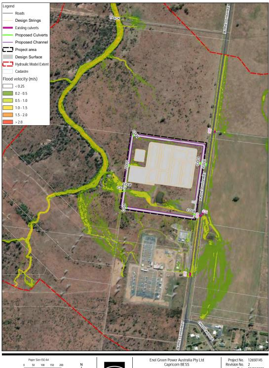
Post-Developed site conditions 10% AEP storm event Flood Velocity (m/s)
