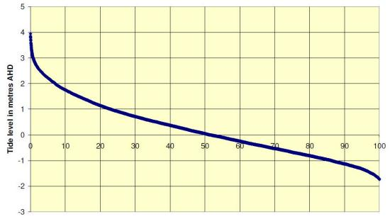
Figure 2. CSIRO modelled tide level duration curve.
