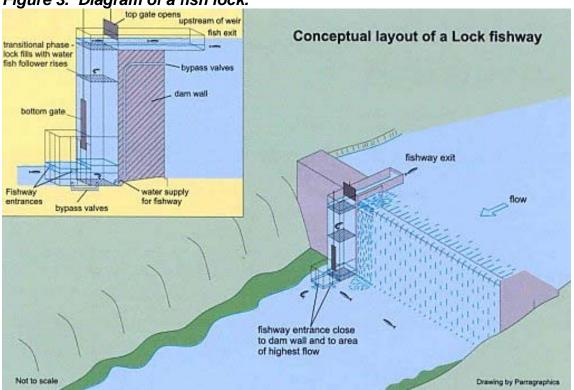
Figure 3. Diagram of a fish lock.
