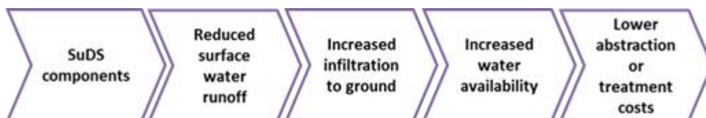
Figure 35 Suds Infiltration Cycle - typical (SUSDrain)
