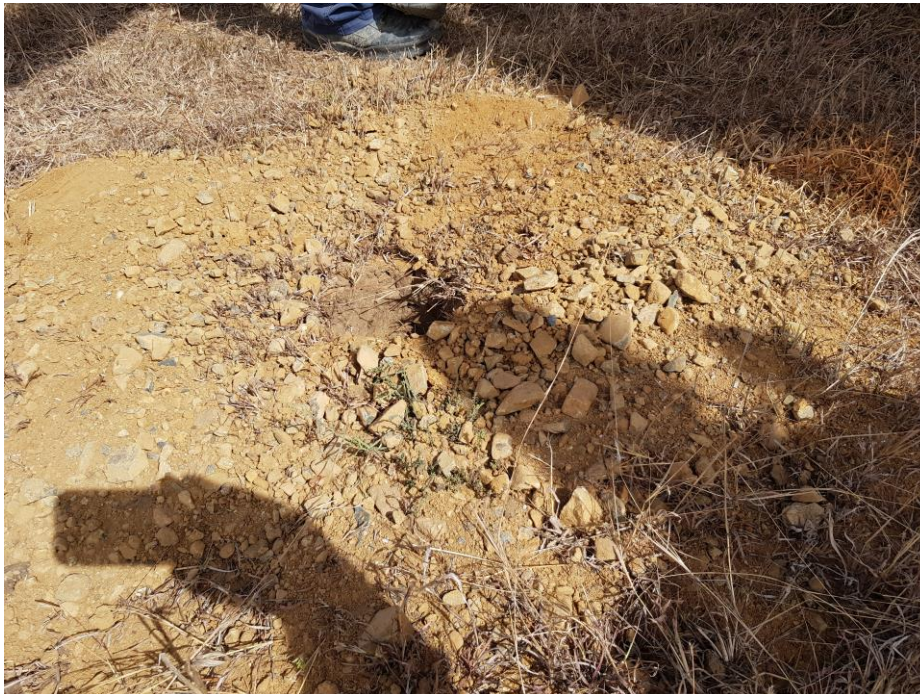
Figure 3-3 Rounded to sub-rounded fine to coarse grained and cobble sized material recovered from BH06. Note larger clasts likely rubbed during drilling causing angular surfaces.
