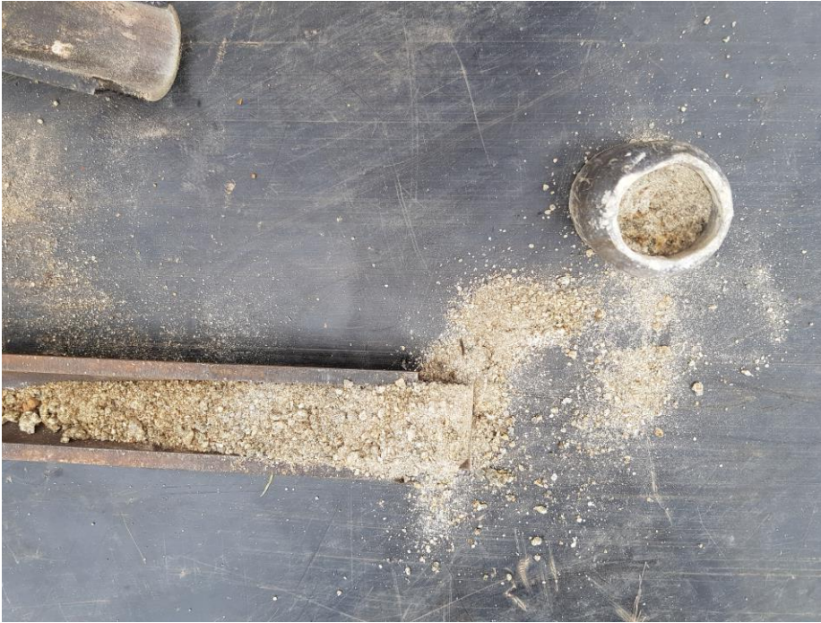
Figure 3-4 Decomposed to extremely weathered granodiorite recovered from BH05 in 3.0m SPT (N=R)
