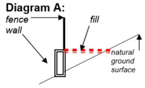
the wall is constructed ON the natural ground surface the wall is to retain fill placed behind the wall the fence is to be constructed on top of the wall
