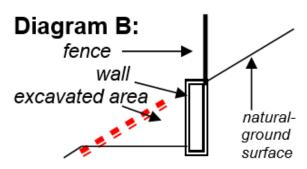
the natural ground surface is excavated the wall is restraining the excavated area the fence is to be built on top of the wall the fence is constructed on the natural ground surface level
