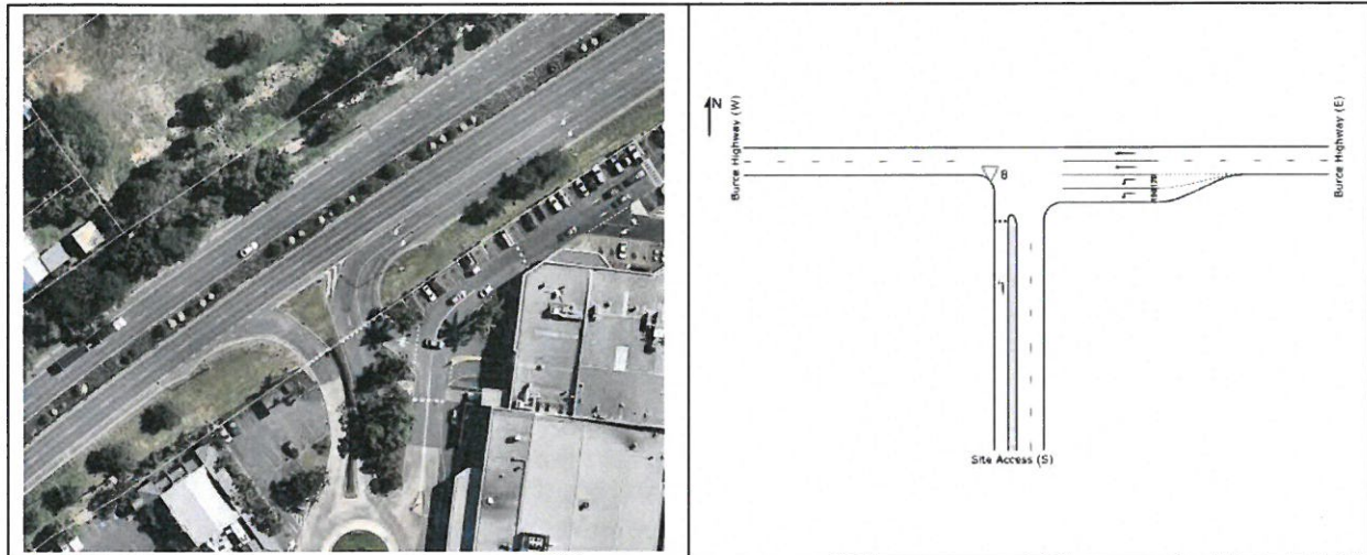
Figure 5-11 Current and SIDRA Assessed Layout – Bruce Highway / Left in Left Out Intersection
