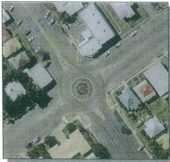
◀ Figure 34: Campbell Street and Archer Street intersection HV swept paths Truck and Dog Trailer only
