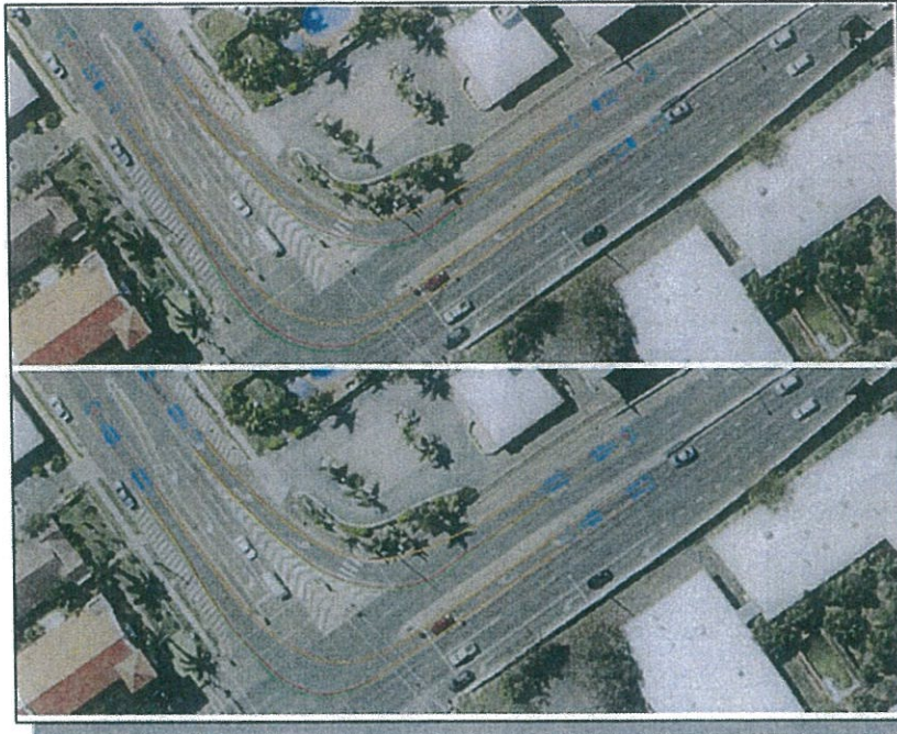
◀ Figure 19: Bolsover Street and Bruce Highway intersection HV swept paths Top: Truck and Dog Trailer, Bottom: Semi Trailer
