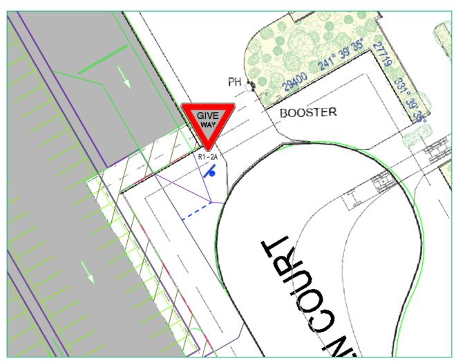
Additionally, the proposed development egress point has been provided with give way line marking and a give way sign to ensure priority is given to vehicles already on Kiln Court. The swept path assessment for the proposed driveway location has been amended to illustrated that the bus / refuse collection vehicle will not impend vehicles from the adjacent development.
