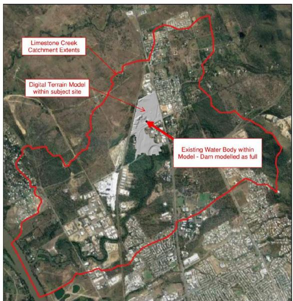
Figure 4: RNAU Model Components (Source: provided RNAU TuFLOW, files - Mapped in QGIS)
