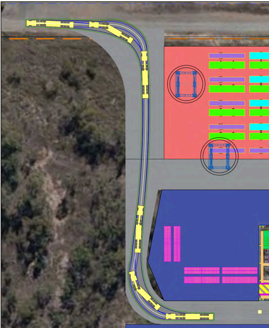
Figure 4.5: Heavy Vehicle Manoeuvring Site Exit (Werribee Street)
