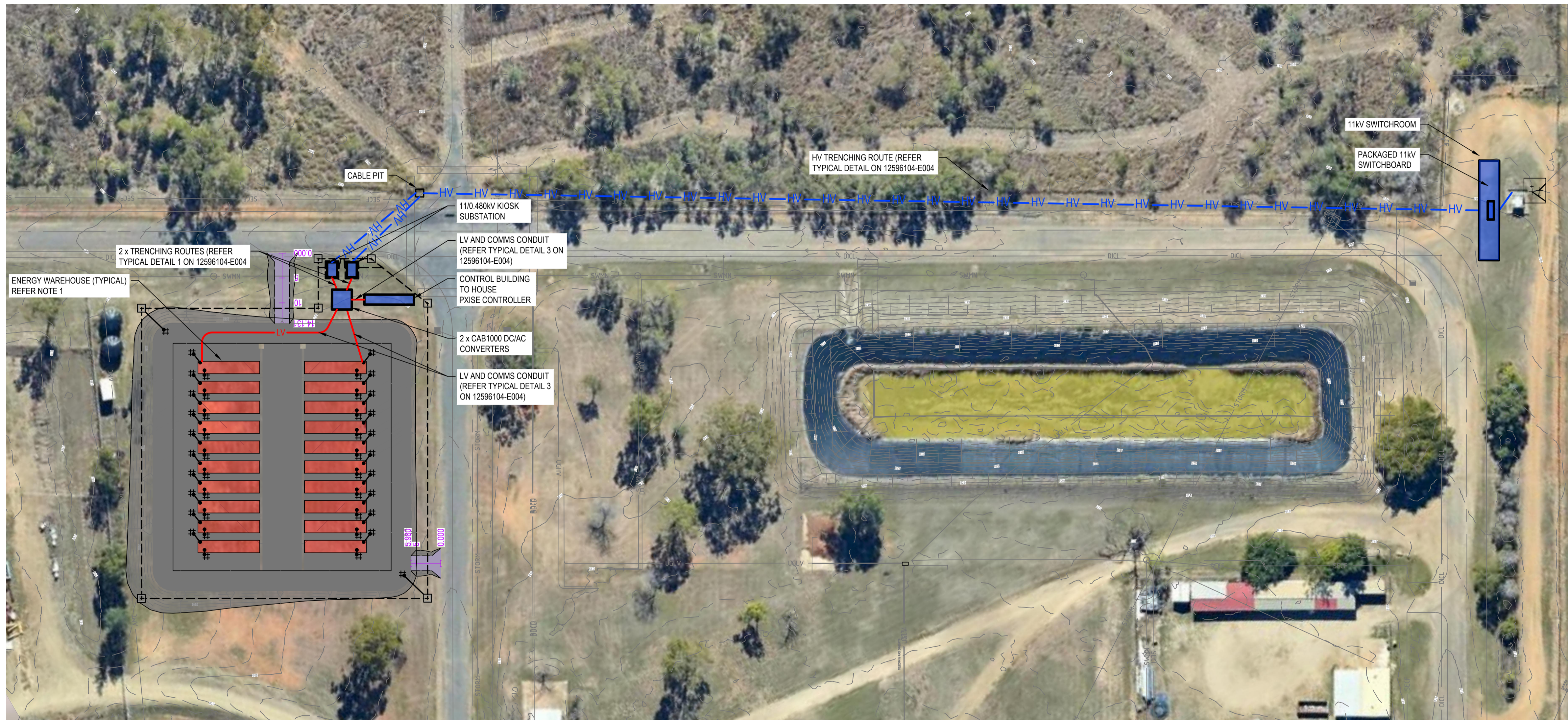
ELECTRICAL CONDUITS AND TRENCHING ROUTES SCALE 1:500
