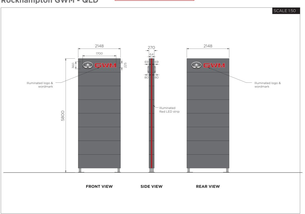
3mm Dark Grey clad to internal frameworks
