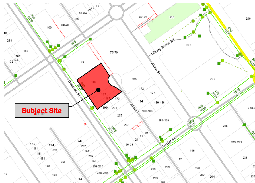
Figure 2 - Existing Stormwater Infrastructure – Shown in Green (Source: RRC Mapping)
