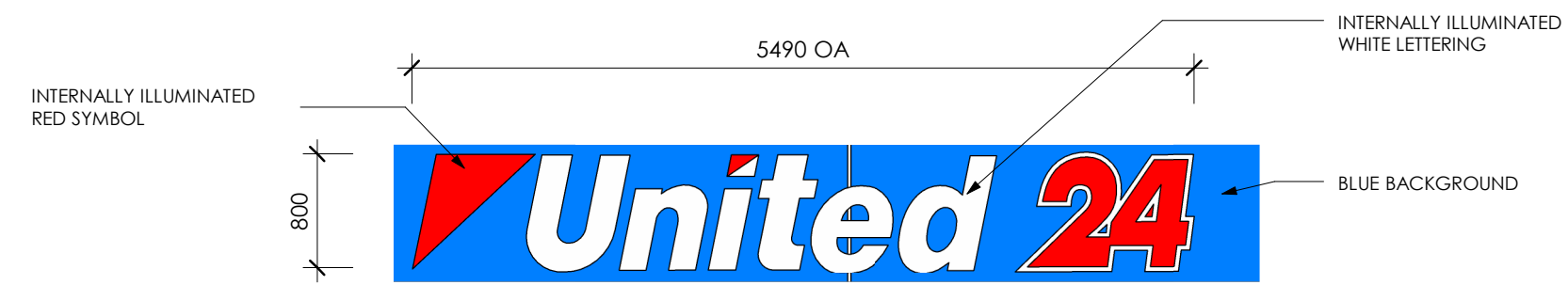
3 SIGNAGE ELEVATION - PETROL FASCIA SIGNAGE Scale: 1 : 50
