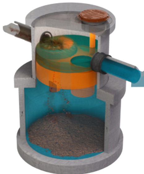
Figure 2 – HumeCeptor® system operation during high flow conditions
