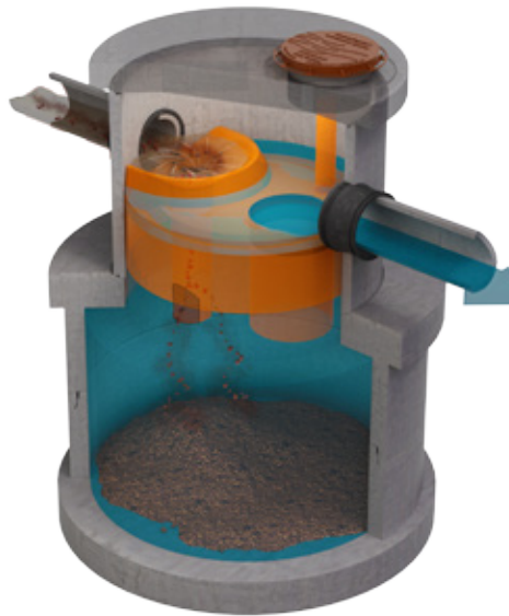
Figure 1 – HumeCeptor® system operation during design flow conditions
