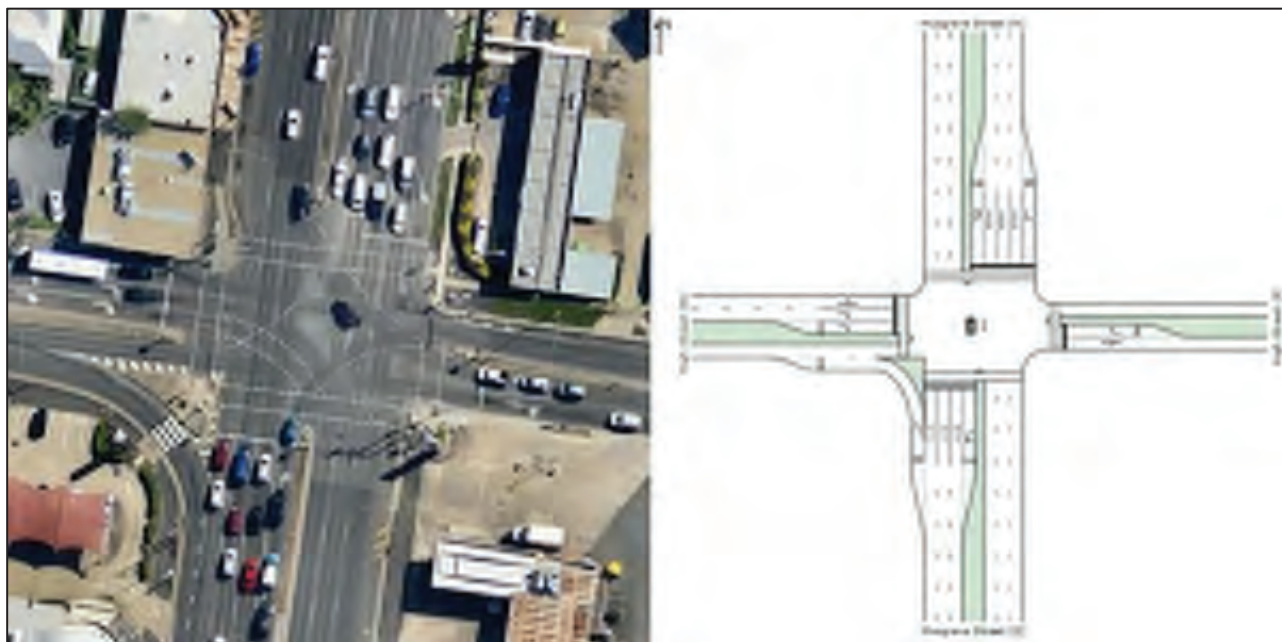
Figure 6-5 Current and SIDRA Assessed Layout – Musgrave Street / High Street Intersection
