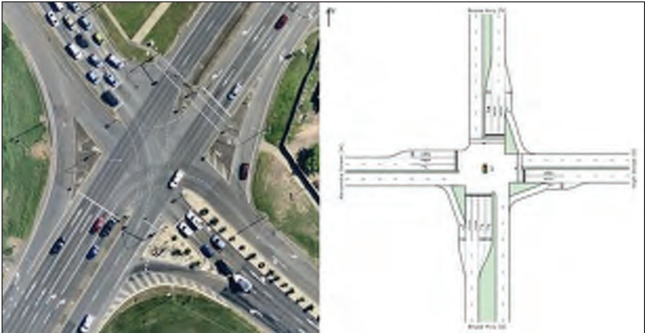
Figure 6-8 Current and SIDRA Assessed Layout – Bruce Highway / High Street / Alexandra Street Intersection
