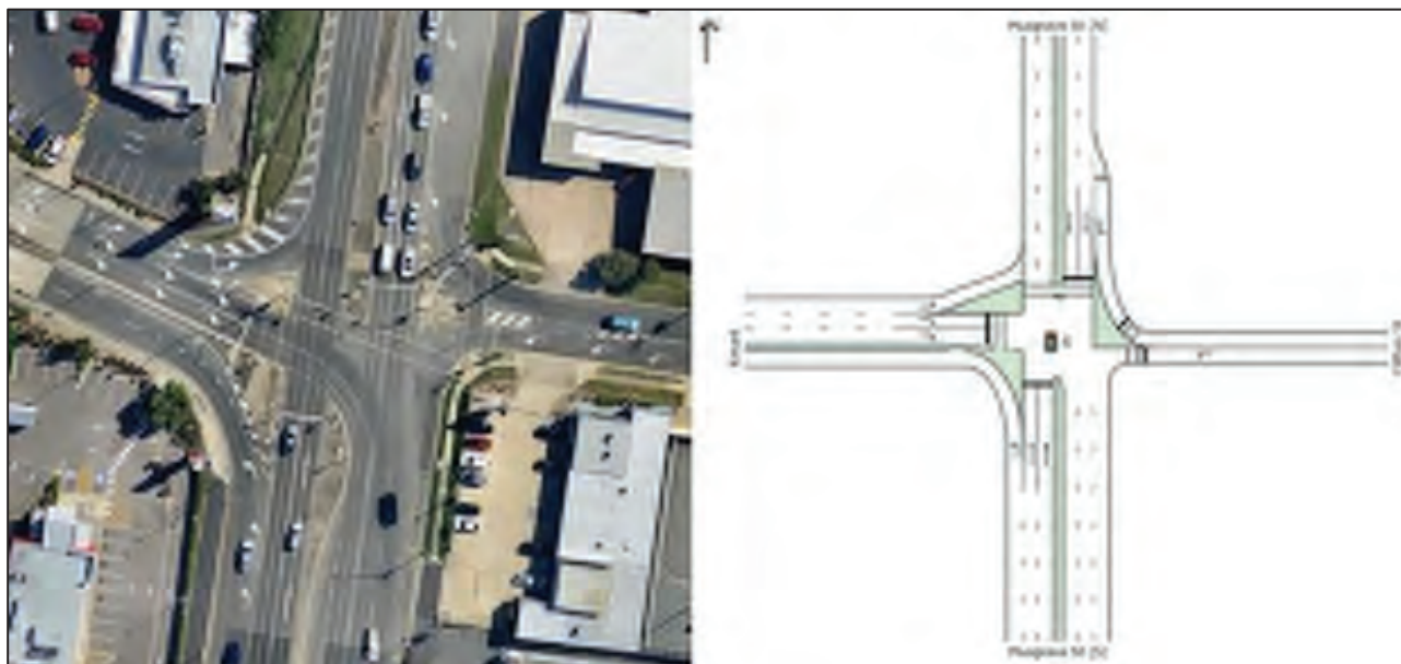
Figure 6-4 Current and SIDRA Assessed Layout – Musgrave Street / Clifton Street Intersection
