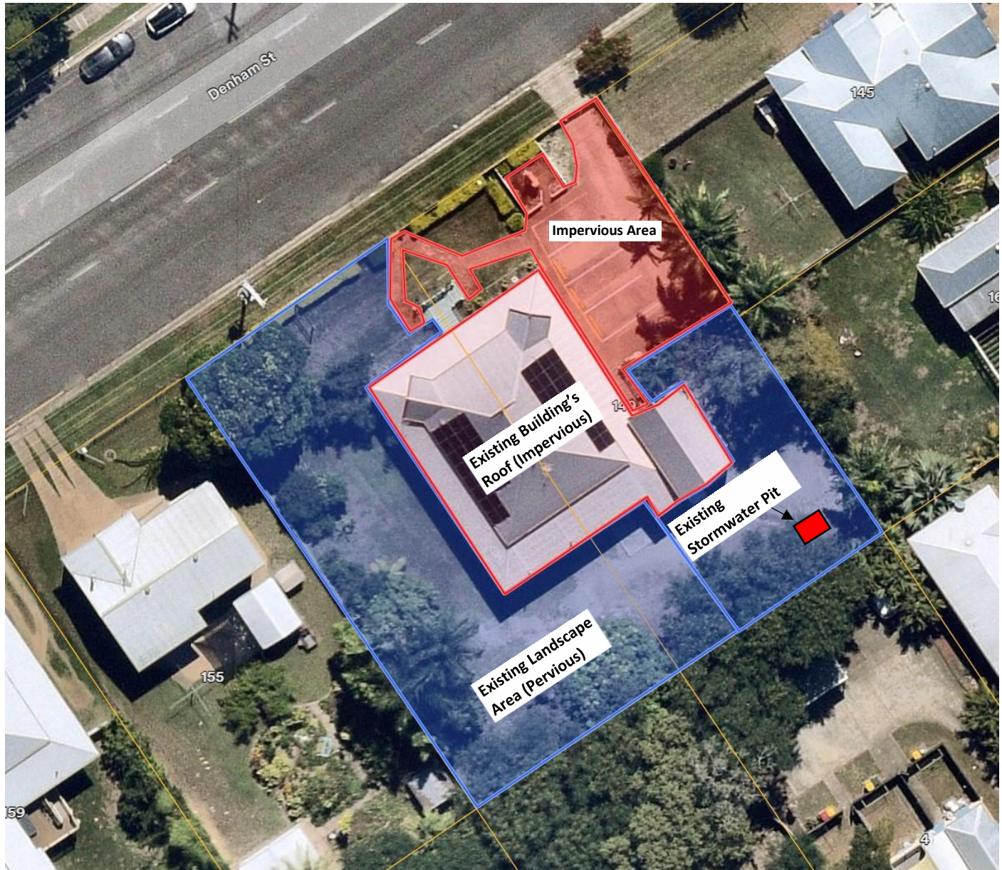
Figure 2: Site plan showing existing site conditions
