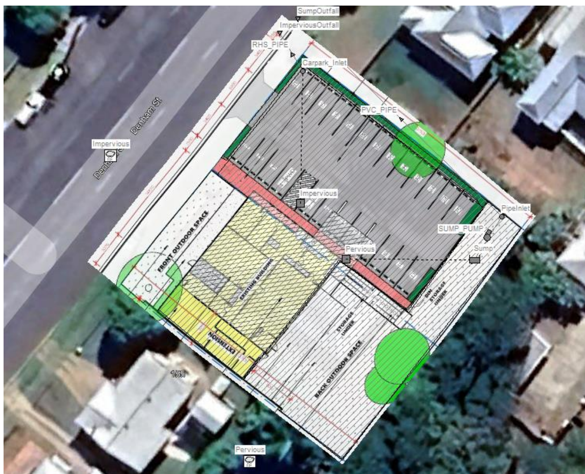
Figure 7: Stormwater management plan layout in EPA_SWMM_5.2
