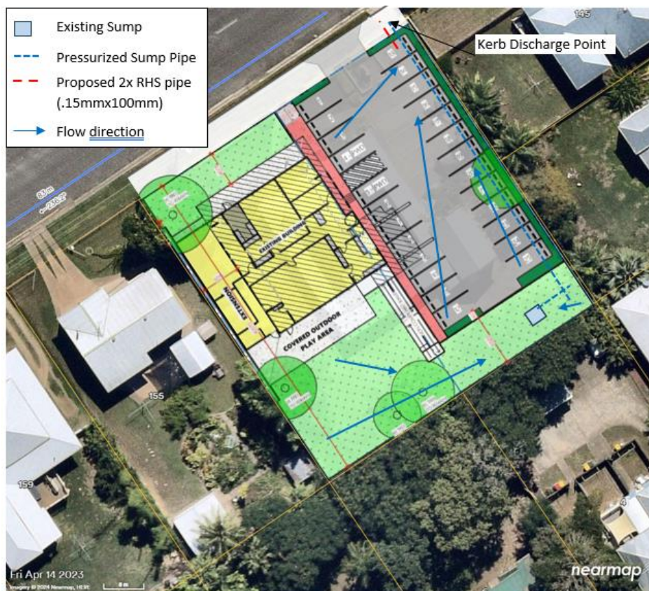
Figure 6: Stormwater management strategy layout plan of Proposed Site Plan
