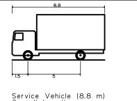
Service Vehicle (8.8 m) Overall Length Overall Width Overall Body Height Min Body Ground Clearance Track Width Lock-to-lock time Curb to Curb Turning Radius
