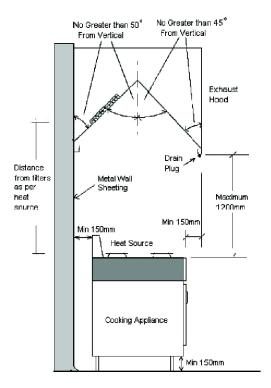
Figure 6. Example plan of a mechanical ventilation system
