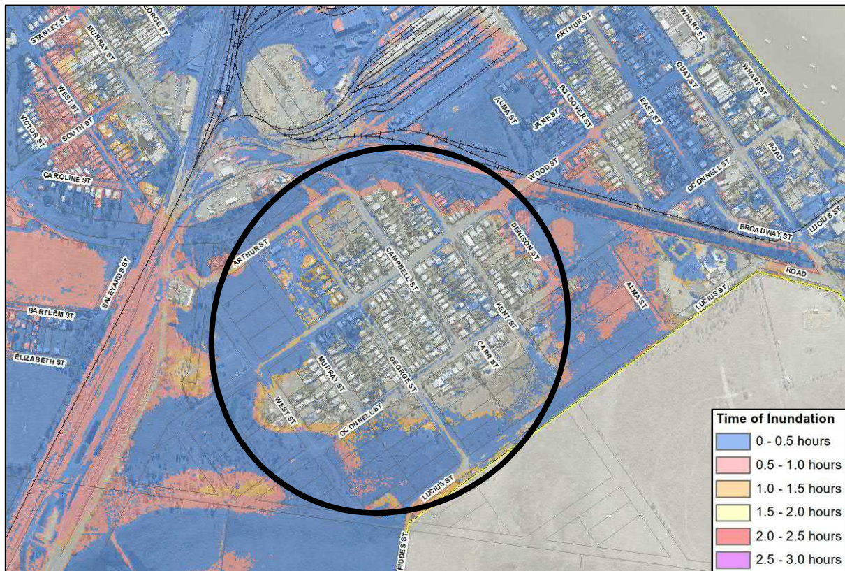
Figure 25 Isolated Area – Depot Hill area (Note: PMF flood extents shown)
