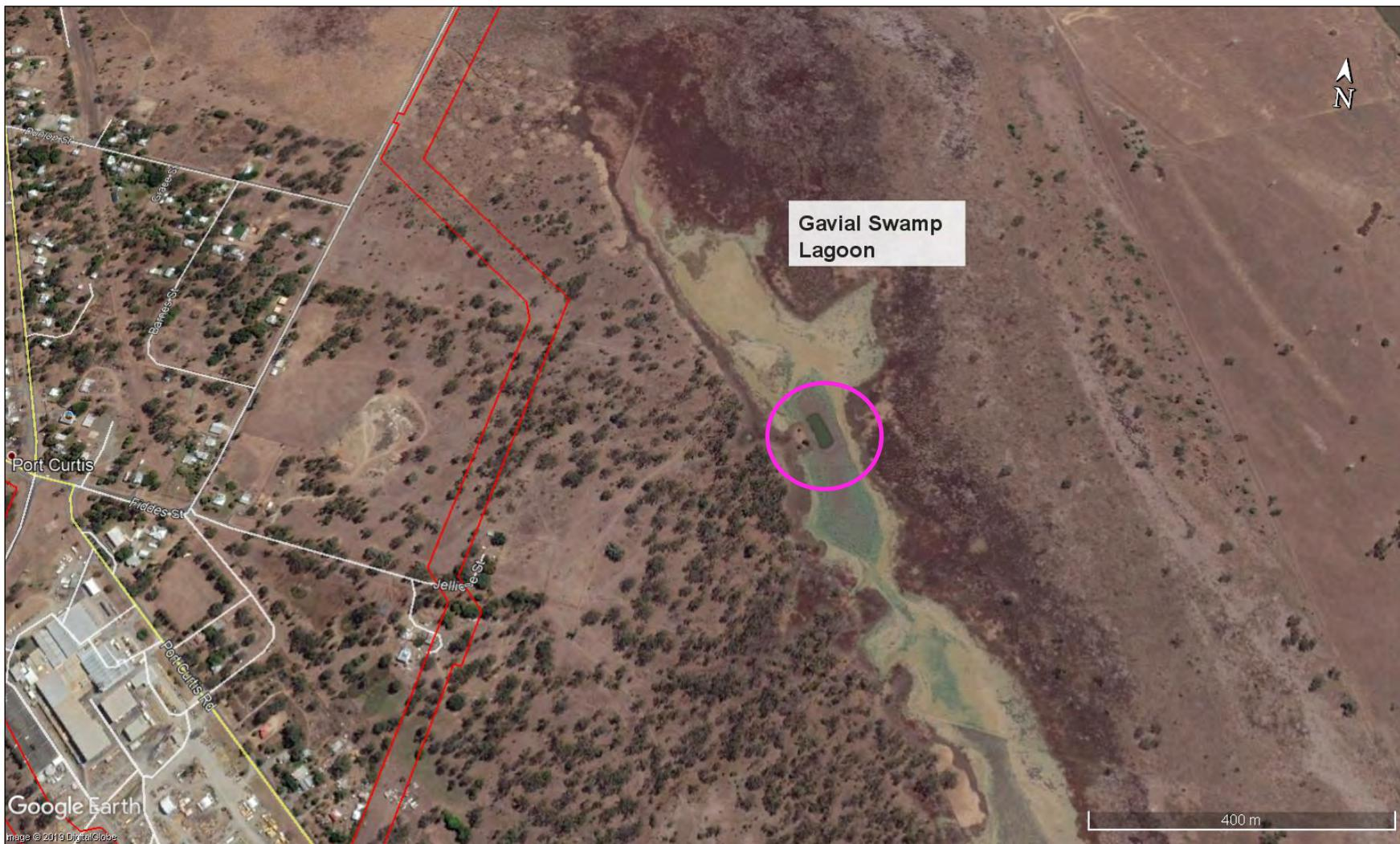
**Figure 7:** Constructed farm dam (circled pink) in the centre of Gavial Swamp Lagoon to increase the period of inundation for cattle drinking water (note; the small vegetated island adjacent to the dam formed excavated material)
