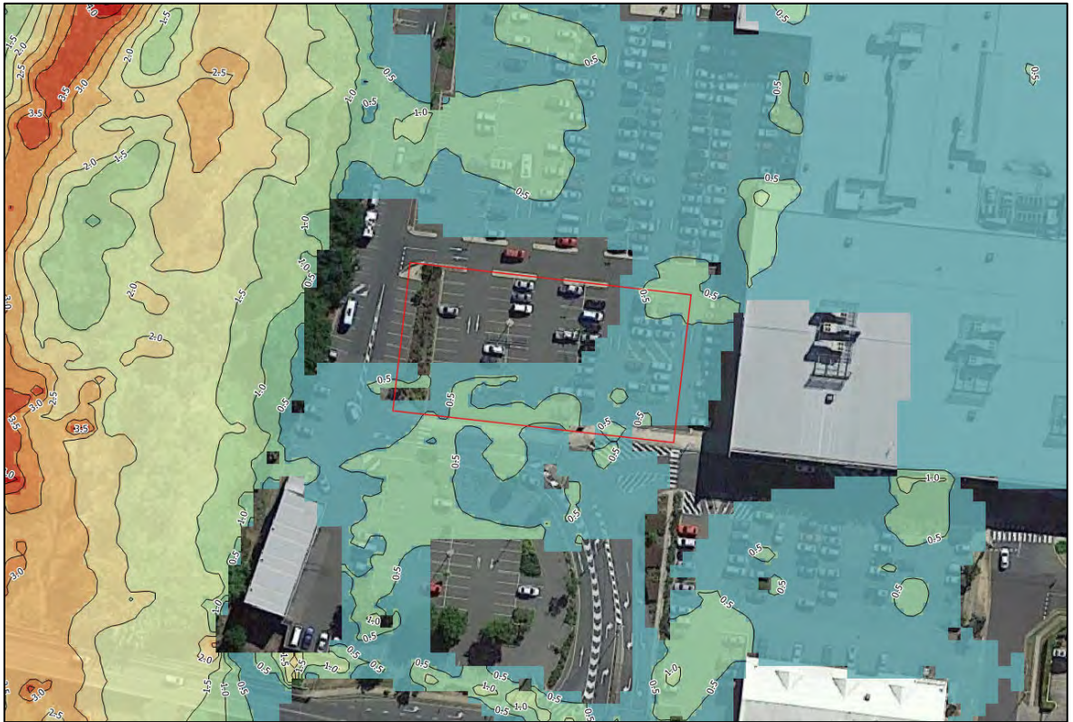
Figure 5.5 – Existing 1% AEP Velocities (m/s)
