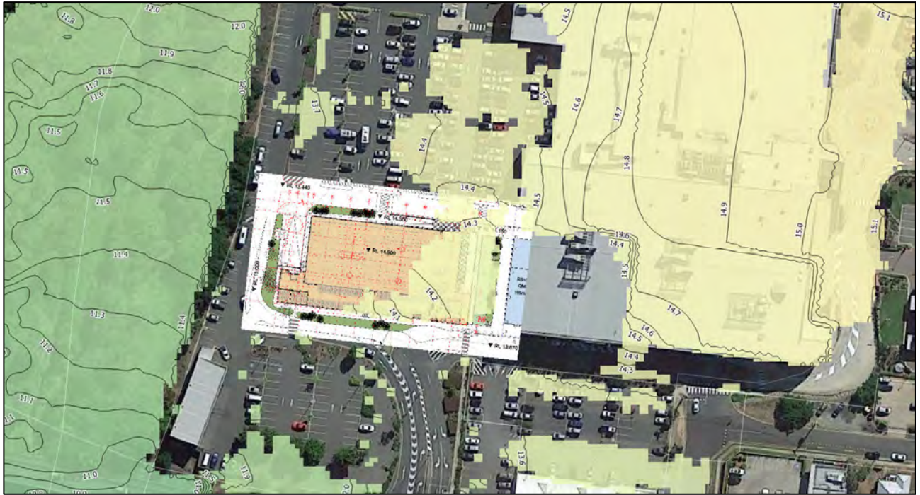
Figure 3.1 – 1% AEP Flood Levels (metres AHD)
