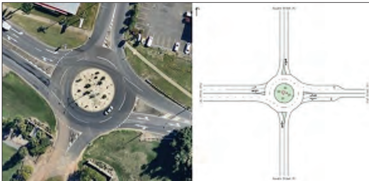
Figure 6-7 Current and SIDRA Assessed Layout – High Street / Aquatic Place Intersection
