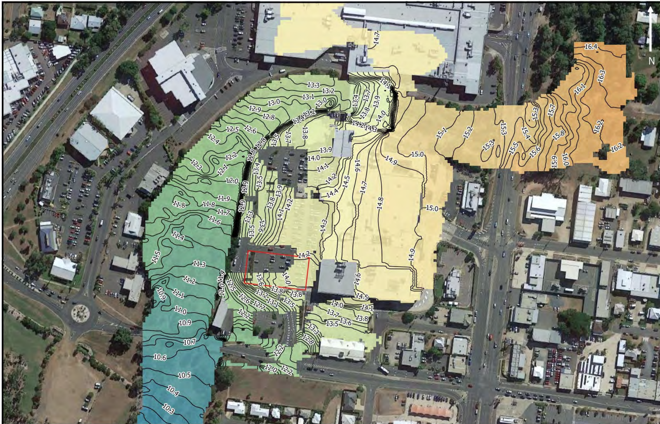
Figure 3 Existing 1% AEP Flood Contours (m AHD)
