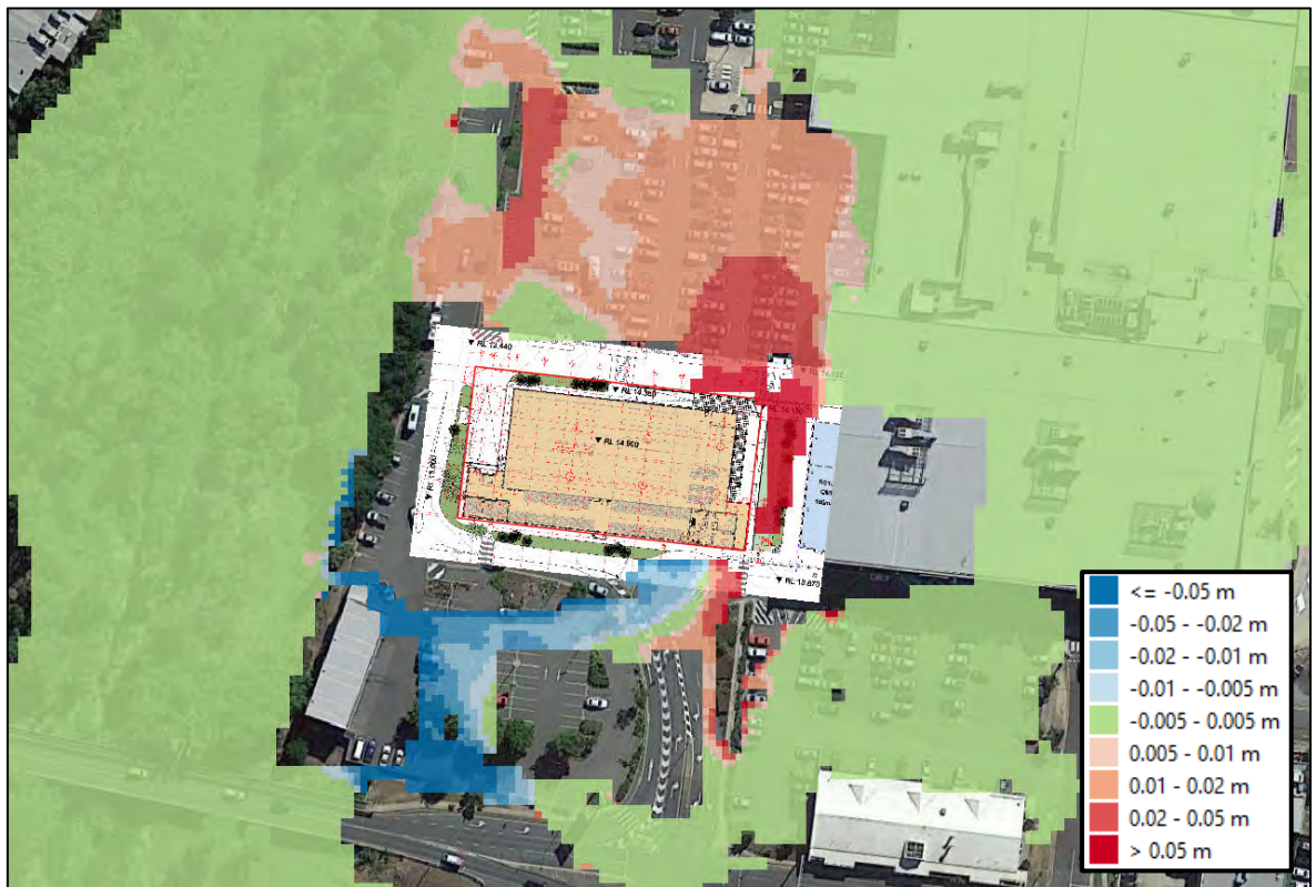
Figure 5.12 – Afflux Impacts Plot (metres)
