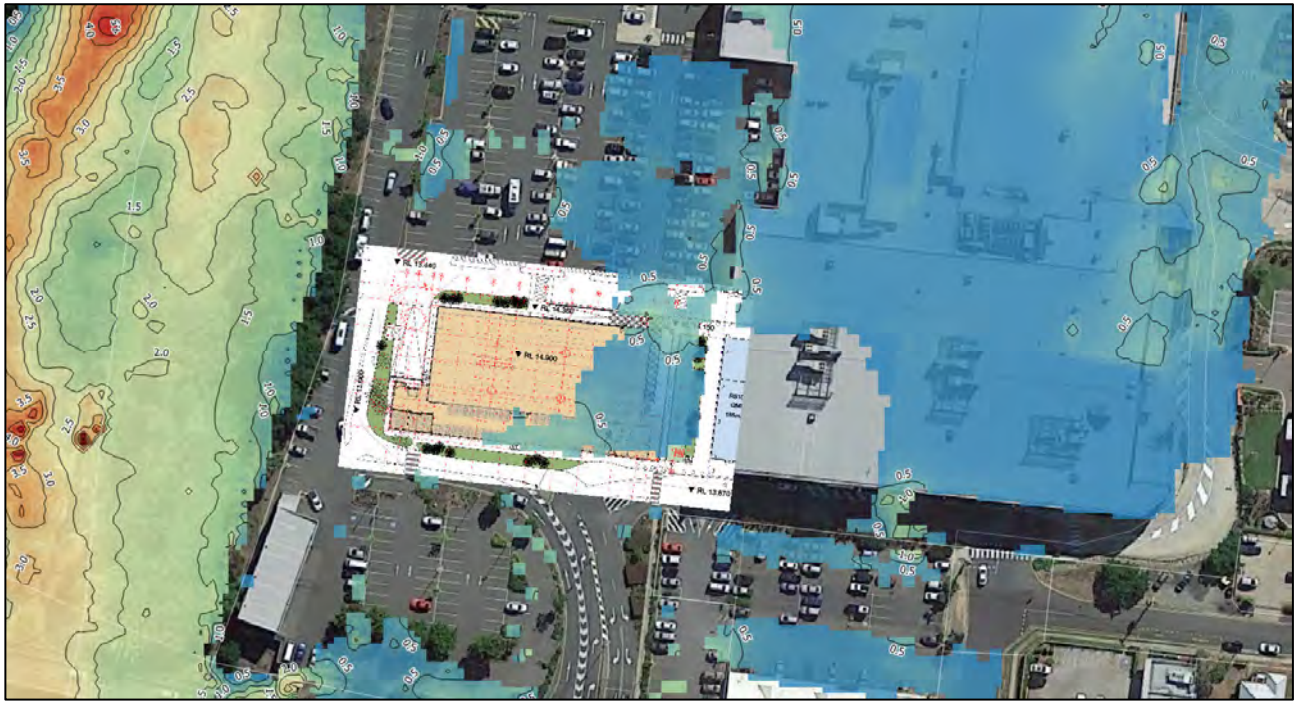
Figure 3.3 – 1% AEP Flood Velocities (m/s)
