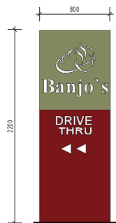
7 SGN2-7 - T2 ILLUMINATED DIRECTIONAL SIGNAGE 1: 20
