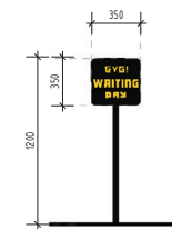
8 SGN1-13 - T1 ILLUMINATED DIRECTIONAL SIGNAGE 1 : 20
