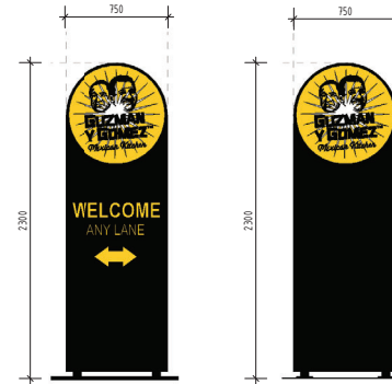
3 SGN1-9 - T1 ILLUMINATED DIRECTIONAL SIGNAGE 1 : 20
