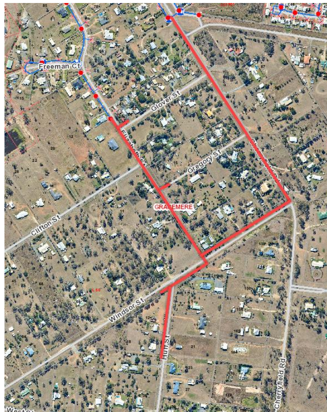
Figure 1. Aerial image showing new water mains (red) constructed in southern Gracemere.
