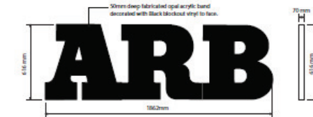
Halo Illuminated acrylic Letters - Front &amp; Side View
