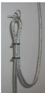
Fig. 5. Cable installation example
