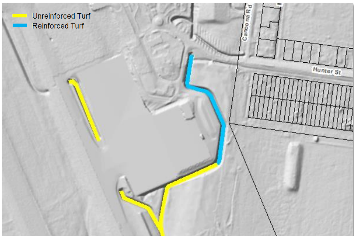
Figure 5 Channel Scour Treatment Overview
