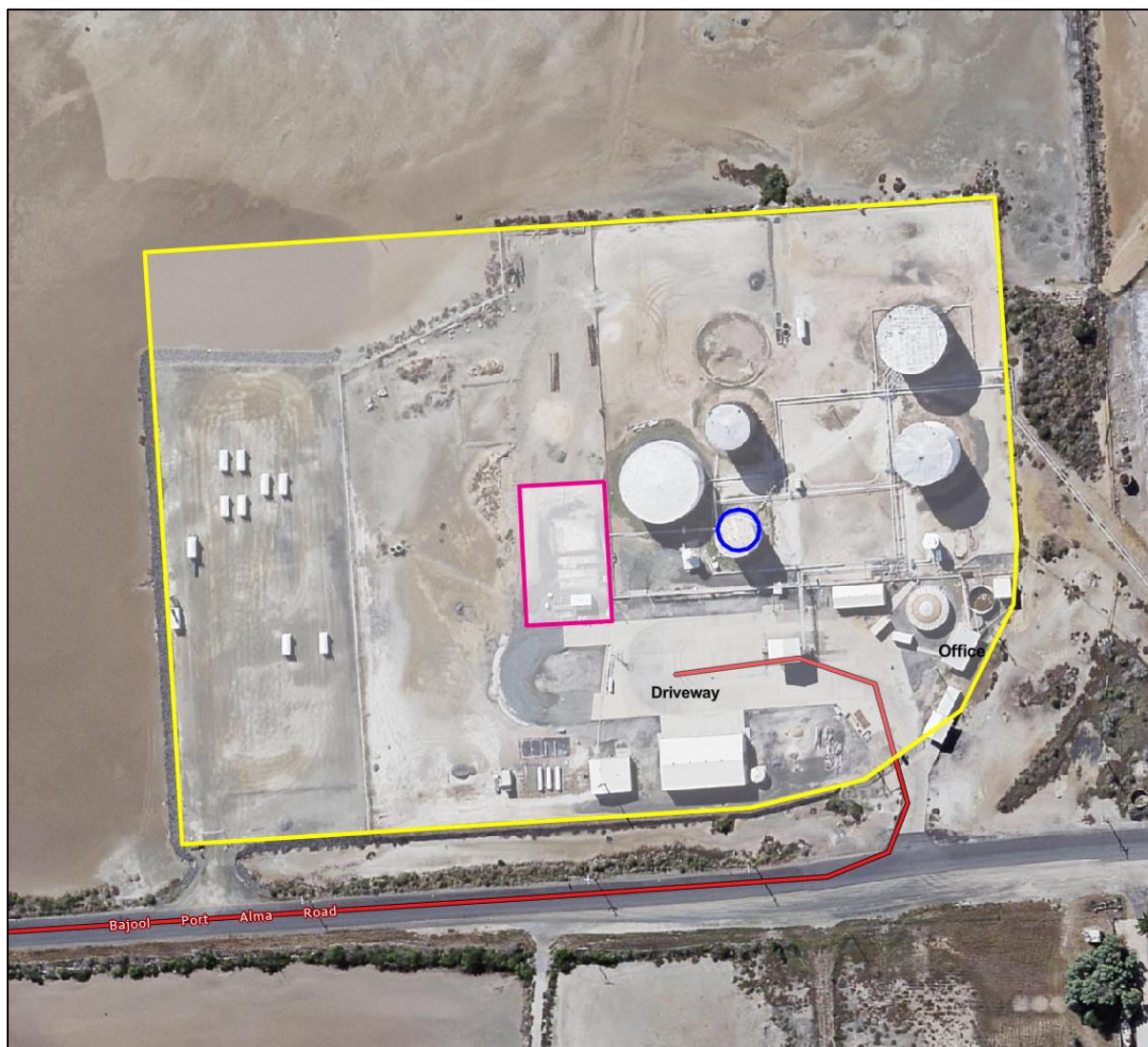
Figure 6. Indicative location for the proposed UCO processing facility is shown by the pink polygon. The existing bulk storage tank that will be used to store processed UCO is circled blue. Trucks delivering UCO will enter the driveway, follow the turning path before parking adjacent to the UCO processing area for unloading.
