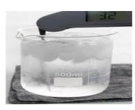
Cold calibration is a safer method of thermometer calibration than hot calibration as there is less risk of getting burnt.
